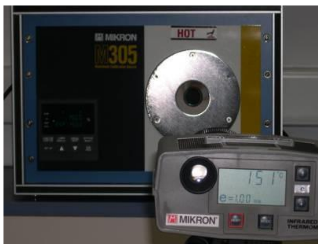
Figure 61. IR sensor calibration using a black body.
