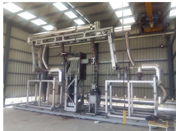
Figure 16. Schematic diagram of the REPA test loop at PSA (a) and north view of the test facility with two flex-hoses mounted for testing (b).
