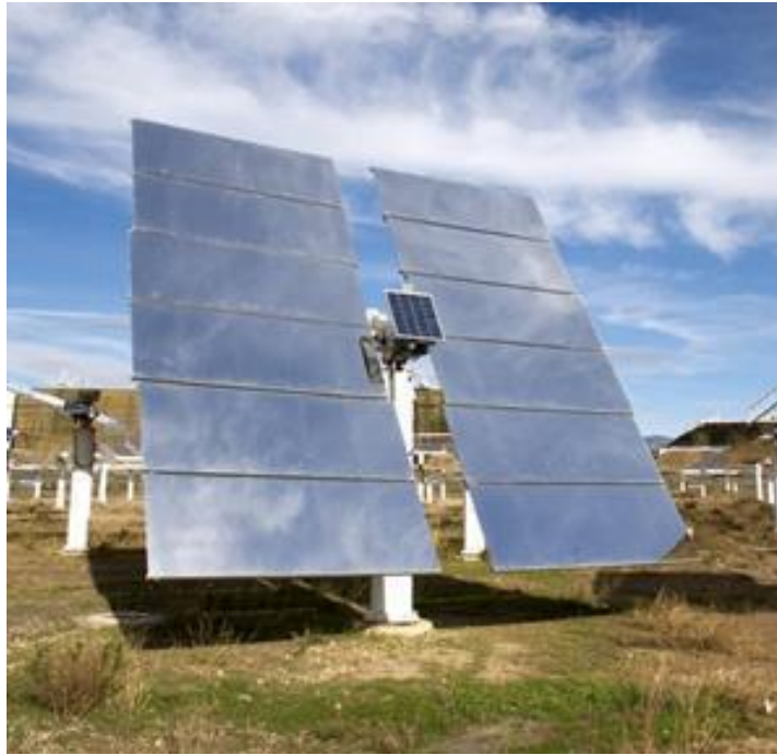
Figure 20. An autonomous heliostat in the SSPS-CRS field.
