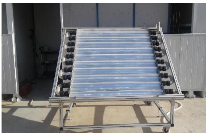
Figure 43. View of 2 m 2 -CPC coupled to Electro-Fenton pilot plant (ELECTROX).
