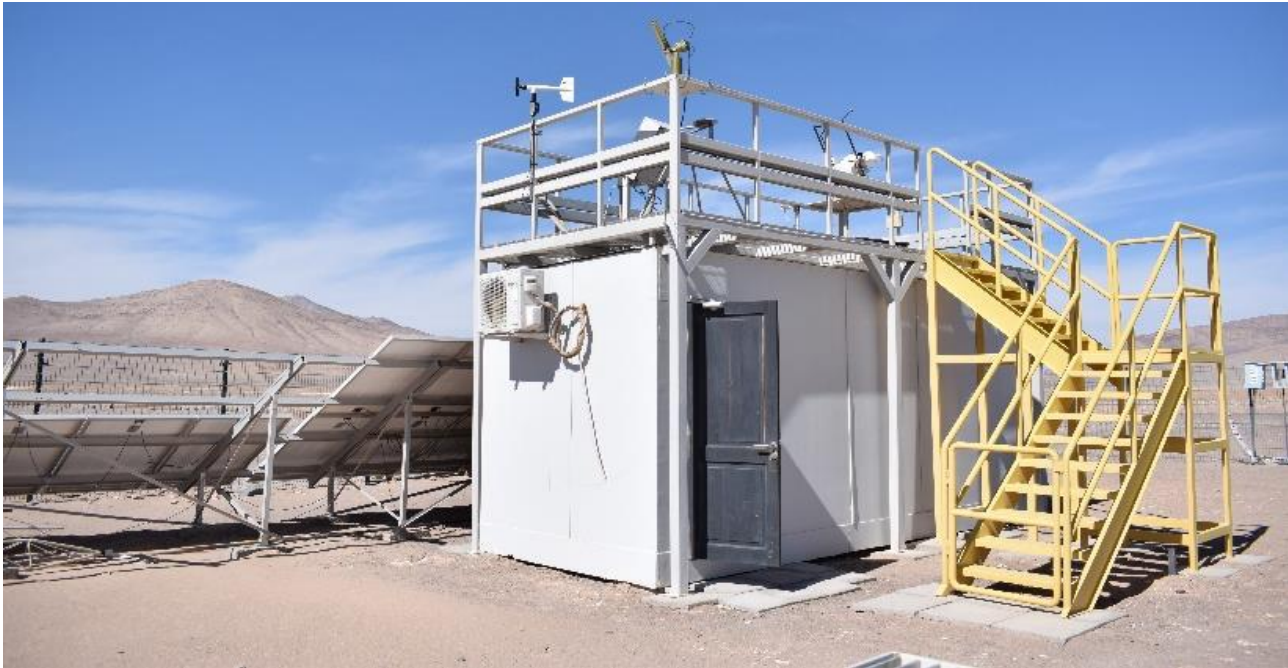
Figure 90. Weather station at the Plataforma Solar del Desierto de Atacama (PSDA) in Antofagasta (Chile). The station is equipped with a large variety of instruments ranging from atmospheric parameter measurements to solar resource measurements, including instrumentation for characterizing atmospheric aerosols and components, visibility sensors and size distribution of airborne particles.
