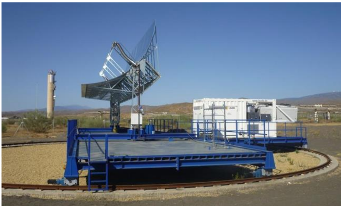
Figure 15. Side view of KONTAS test bench and the heating/cooling unit (right side).
