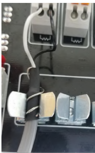
Figure 18: BOM cable inserted into 360° shield connection
