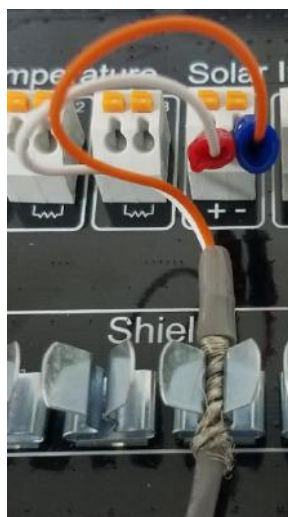
Figure 20: Solar irradiance sensor shield connection
