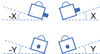
Figure 5.2A Tilt angle (-180 to 0°) and (0 to 180°) Roll angle (-180 to 0°) and (0 to 180°)
